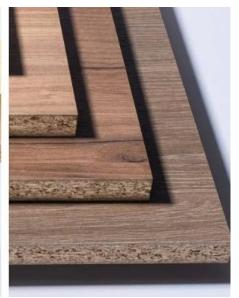
Particle board is widely used in furniture manufacturing, especially as a substrate for cabinets, bookshelves, desks, and TV cabinets. Its lightweight properties also make it an ideal choice for indoor partitions and soundproof walls. Particle board is commonly used as a material for the lower floors and interior decoration projects, such as doors and decorative panels.
