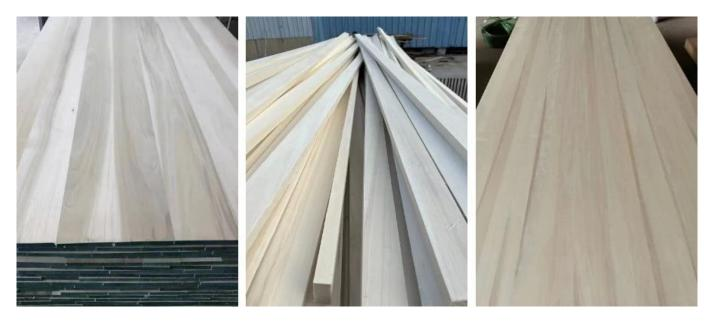
Poplar wood is often used in the construction industry for components such as beams, purlins, and ceilings. Its delicate texture and moderate hardness make it a good material for furniture manufacturing, allowing for the production of both aesthetically pleasing and stable furniture products.
